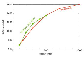
Fig. 6. The GEM trip voltage, and the relative gain at a constant GEM voltage, are shown as a function of gas pressure. Both nearly scale with  $\sqrt{\text{pressure}}$
