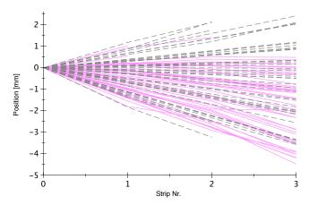
Fig. 5. Electron drift times with respect to the first strip, converted to distances assuming a drift velocity of  $12 \text{ mm/}\mu\text{s}$ . The electrons are released along the tracks of the  $\alpha$ 's. The dashed lines stem from a GEANT4 simulation, the solid, purple lines from the measurement.
