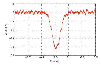
Fig. 7. Amplified signal of  $\approx 5$  MeV  $\alpha$  particles at 500 mbar.
