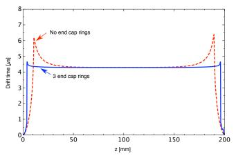
Fig. 11. Drift time of electrons released at -500 V biased cathode wires to the GEM vs. the z-axis, with and without voltage-shaping rings at the end caps.at 10 mm radius. The radii of the cathode cage and of the GEM cylinder are 10 mm and 50 mm, respectively.
